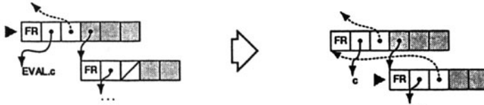
Figure 1: Calling EVAL to reduce a frame node.
