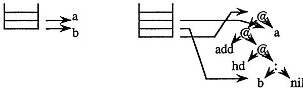
Fig 2.1 A subgraph representing the expression 'add (hd(cons b nil)) a' is constructed. The left part of the figure shows the pointerstack before this operation. Afterwards the top of the pointerstack points to the root of the subgraph just constructed.
